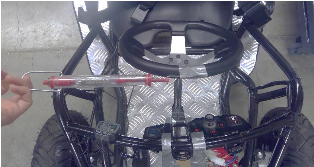
Figure 1. Shows test setup with a force gauge attached to the steering wheel to measure the force necessary to turn the wheel when the cart is at a standstill.
