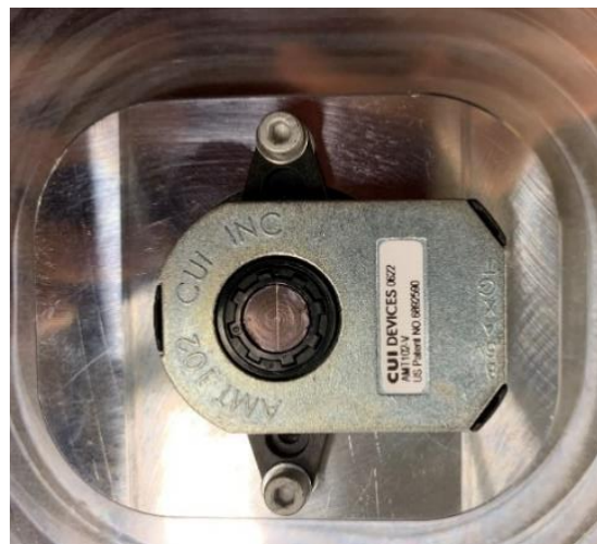
Figure 6. Top View of Gearbox Showing Scribed Centerline on Output Shaft
